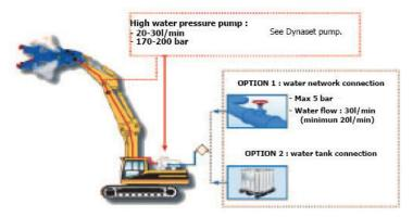
NB: Pump working with the carrier's hydraulic system
